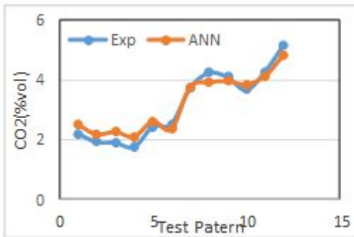
Figure 22: Comparison of experimental CO 2 emission with ANN CO 2 .
