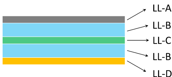
Figure 1: Composition and the stacking sequence of LLDPE layers (five layers) in the film
