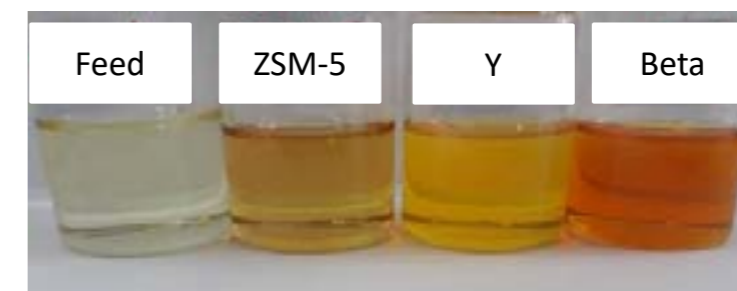
Figure 11. Appearance of liquid cracked product obtained after 210 minutes reaction time
