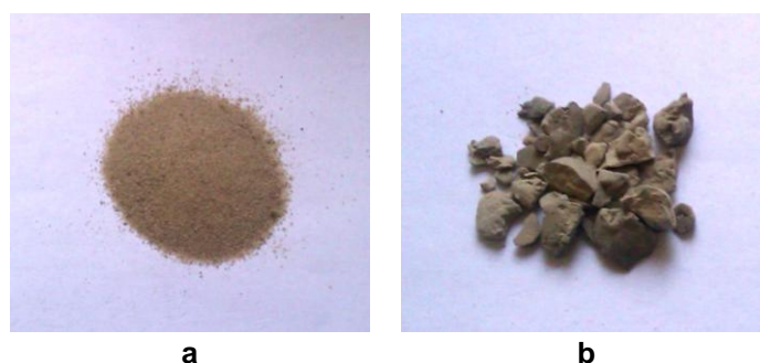
Figure 4. The powdered sandstone (a) and the one with NC hydrogel adsorption (b).
