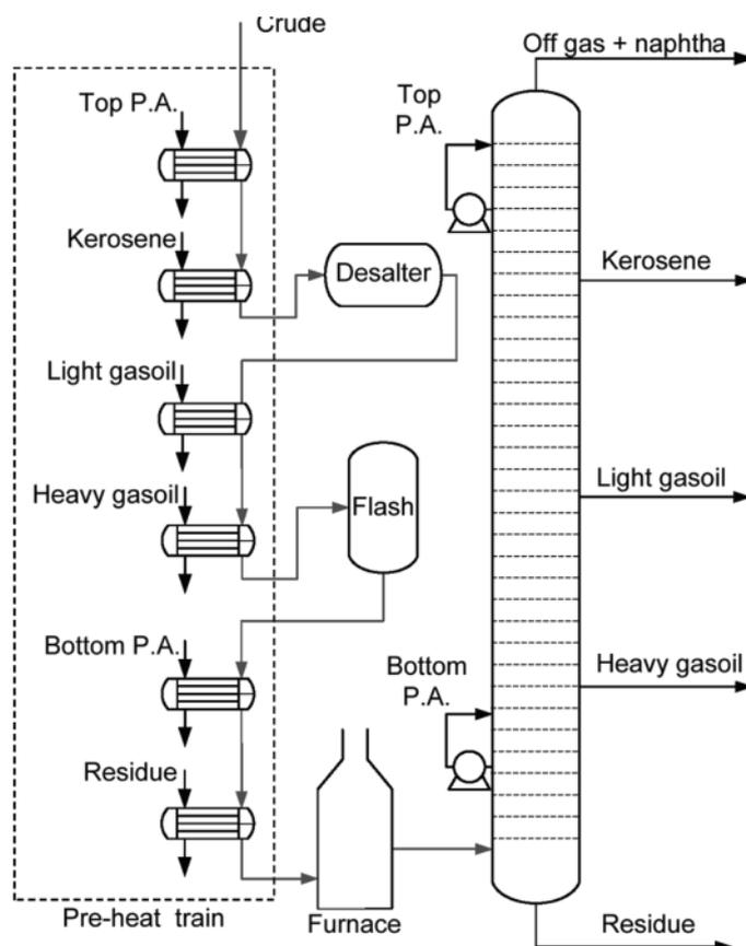
Figure 1. Schematic of a typical Crude Distillation Unit (CDU) including PHTs [4]
