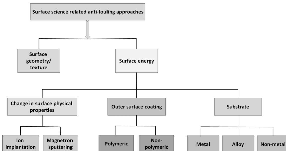
Figure 5. Surface modification methods with anti-fouling properties
