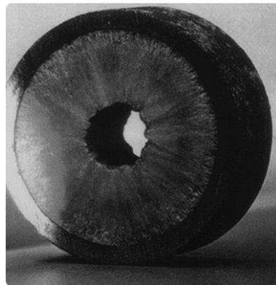
Figure 3. A scheme of wax fouling in pipeline [9]
