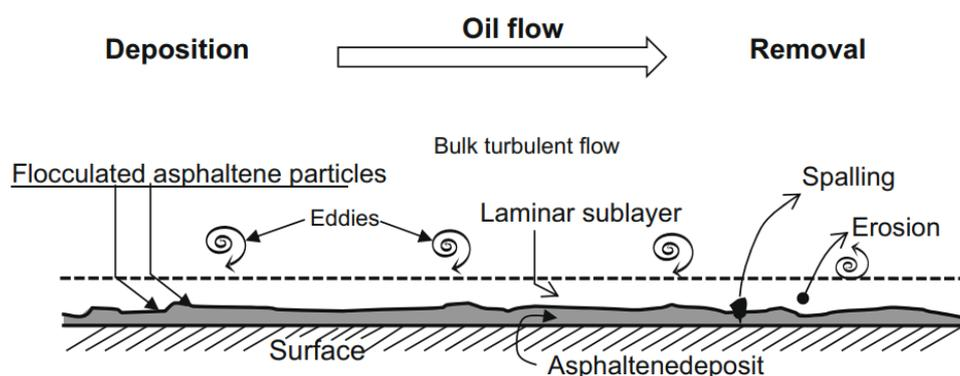
Figure 4. A schematic of Asphaltene deposition and removal steps [20]
