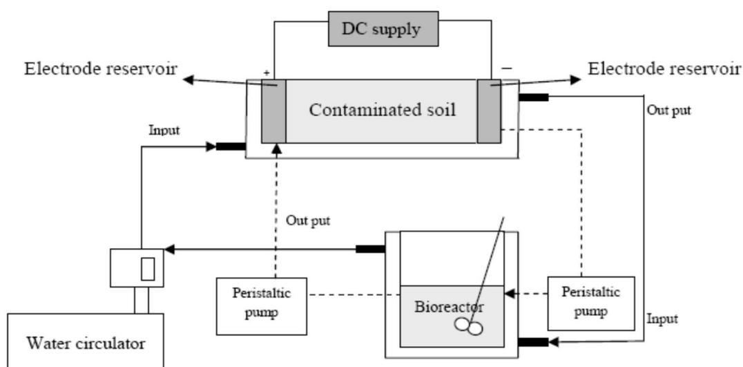
Figure 1. Schematic diagram of EK – bioremediation cell
