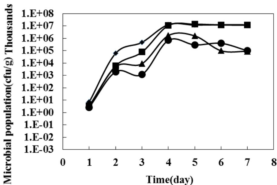
Figure 3. The variation of microbial population in anode (◆), after anode (■), before cathode (▲) and cathode (●) regions of soil during EK – bioremediation with the current densities of  $2.85 \text{ mA}\cdot\text{cm}^{-2}$ .
