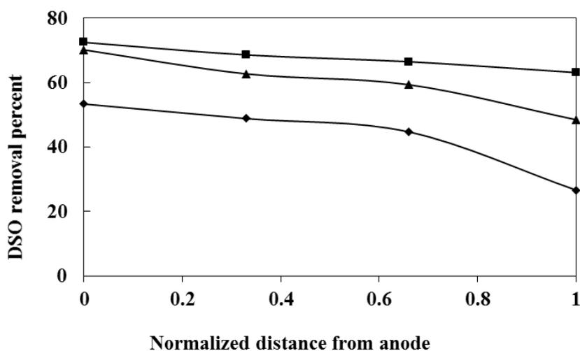
Figure 2. DSO removal percent gradient from anode to cathode in different current densities,  $\blacklozenge$ , 0.6  $\text{mA}\cdot\text{cm}^{-2}$ ;  $\blacktriangle$ , 2.85  $\text{mA}\cdot\text{cm}^{-2}$ ;  $\blacksquare$ , 2.42  $\text{mA}\cdot\text{cm}^{-2}$ .
