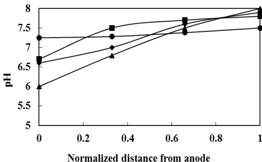
Figure 4. The pH gradient from anode to cathode in different current densities after 2 days during EK – bioremediation process, ◆, 0.6 mA.cm<sup>-2</sup>; ■, 1.21 mA.cm<sup>-2</sup>; ▲, 2.42 mA.cm<sup>-2</sup>; ●, 2.85 mA.cm<sup>-2</sup>.
