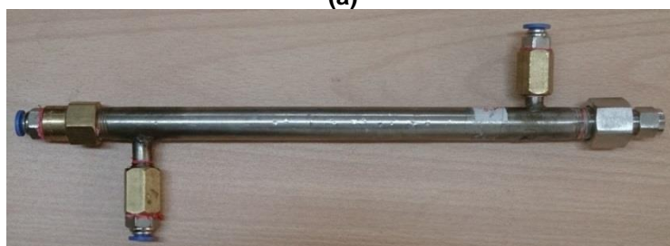
Figure 1: a) Schematic of cross flow ultrafiltration system, T: feed tank, P: pump, PI: pressure gauge, TI: thermometer, M: membrane module. b) Membrane module
